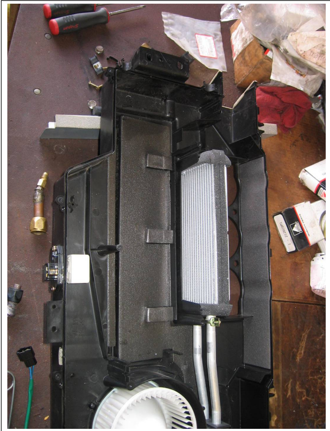
Evaporator box removed and open. Be sure to drill out or uncap the drain tubes.
